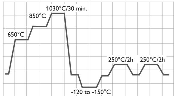
Subzero cooling is only required when demands on dimension stability during use are very high. Received hardness: 52-54 HRC.
