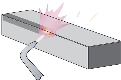
The surface to be hardened is heated continuously by means of a gas flame to approx. 850°C (pale-red colour), followed by cooling in air. The gas flame may be an ordinary oxyacetylene flame. The size of the blowpipe and the temperature of the gas are adapted so that the heating is accomplished in a few seconds.
