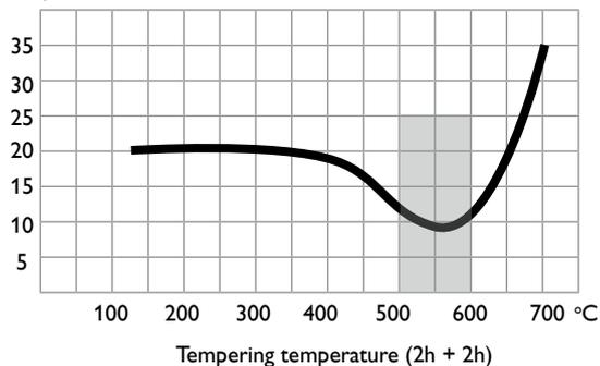
Tempering within the range 500–600°C is normally not recommended due to the reduction in toughness properties.
