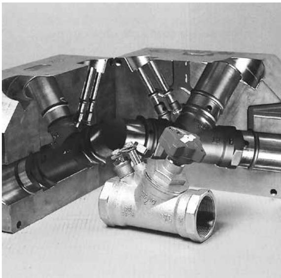
The combination of high temperature strength, temper resistance and thermal conductivity, exhibited by QRO 90 Supreme is unparalleled. Thus QRO 90 Supreme has given improved service life in die casting and extrusion of nonferrous metals and forging and extrusion of steel.
